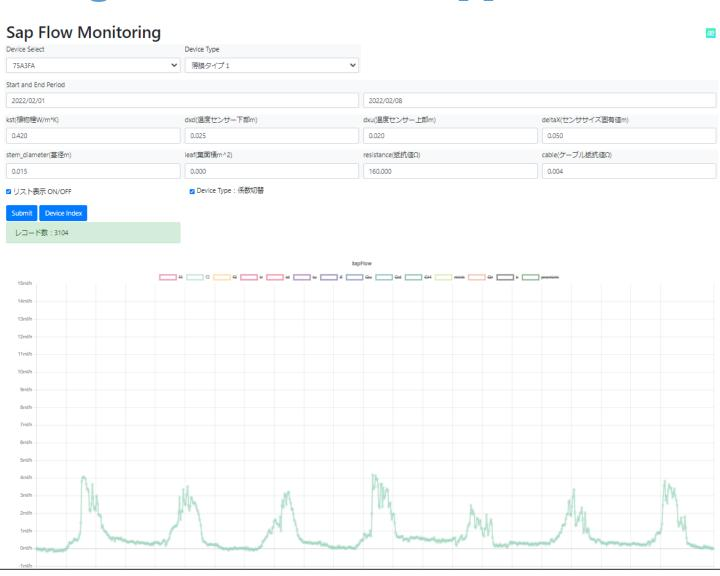
Real-time remote monitoring of sap flow rates is possible by using Skylon application linked to the SigFox cloud. This WEB application is being developed in collaboration with Agrishot and Focus Systems.
